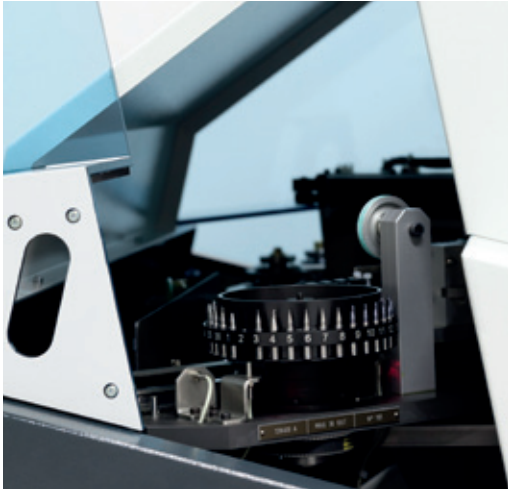
Easy access to the tool magazine, quick manual tool changes using the disc with 36 positions
