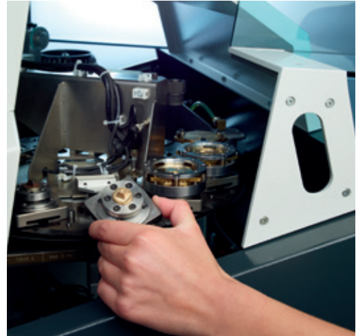
Magazine of 12 pallets on a rotating plate perfectly integrated into the 701S machine
