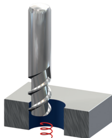
750 rpm x pitch of 0.1 mm => Fz = 75 mm/minute
